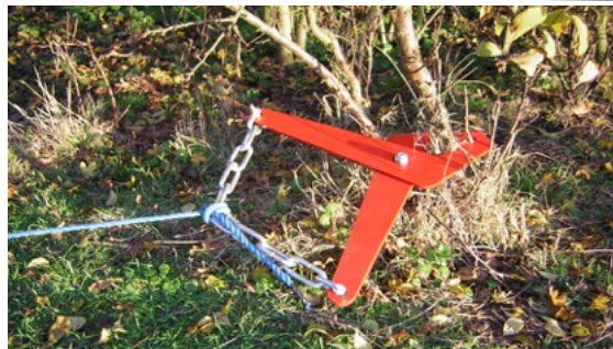
Scrub Puller (left). For pulling out and removing unwanted saplings bushes and scrub. It handles up to 50mm diameter for pulling, lifting and carrying. Ideal for handling and carrying thorn bushes etc. Price £112
